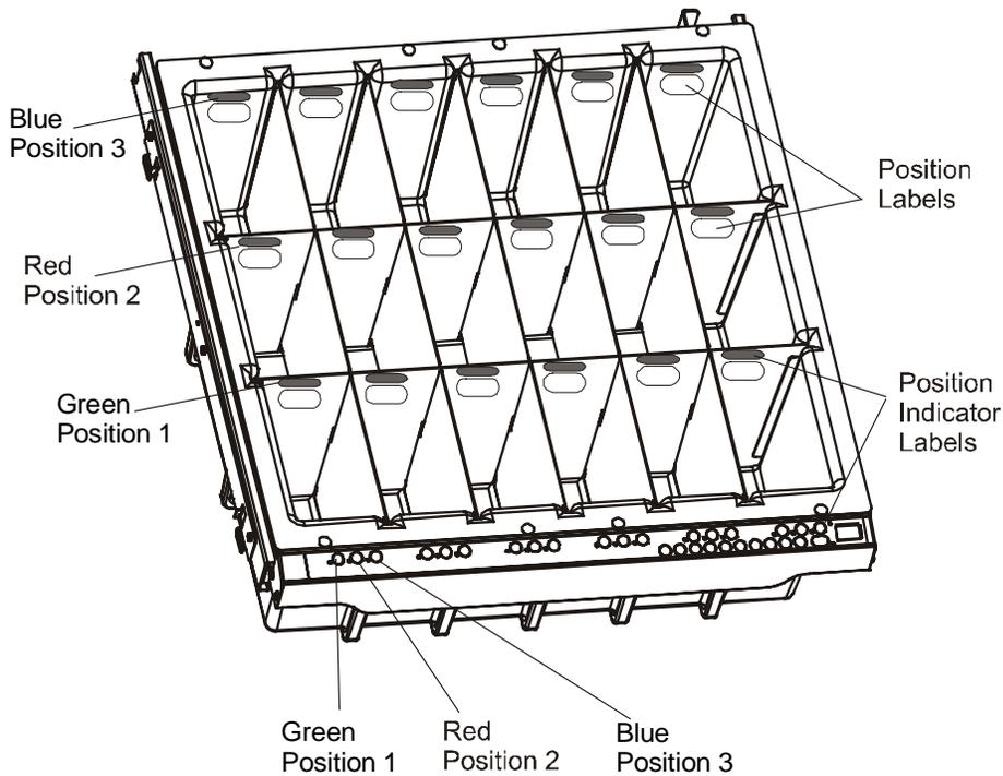
**Figure 2-1 Proper Labeling of a Sliding Shelf**
