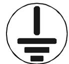
This symbol indicates a protective conductor terminal that is earth grounded.
